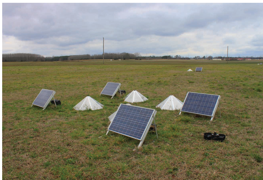
FIGURE 2. Tornado-detecting infrasound arrays, developed by University of Mississippi researchers, incorporate anywhere from five to 10 sensors. (Source: Shea Stewart/University of Mississippi; used with permission.)
